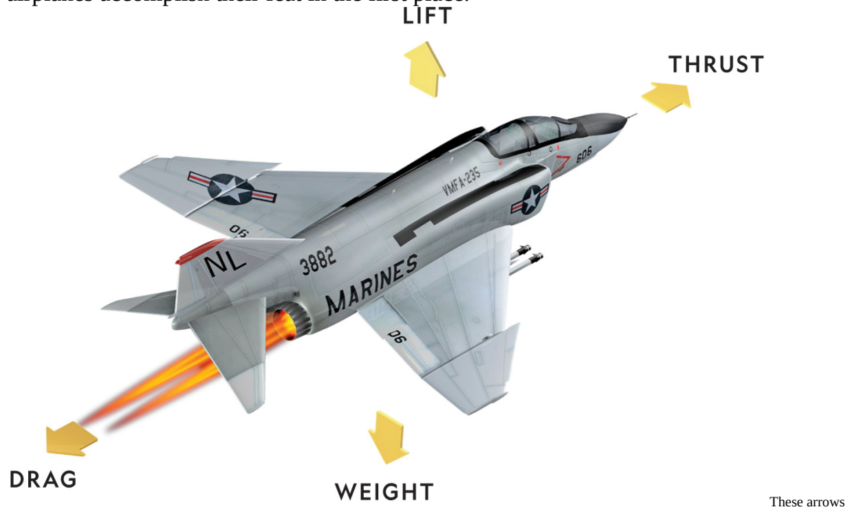
These arrows visualize the forces—lift, weight, thrust, and drag—that act on an airplane during flight.
