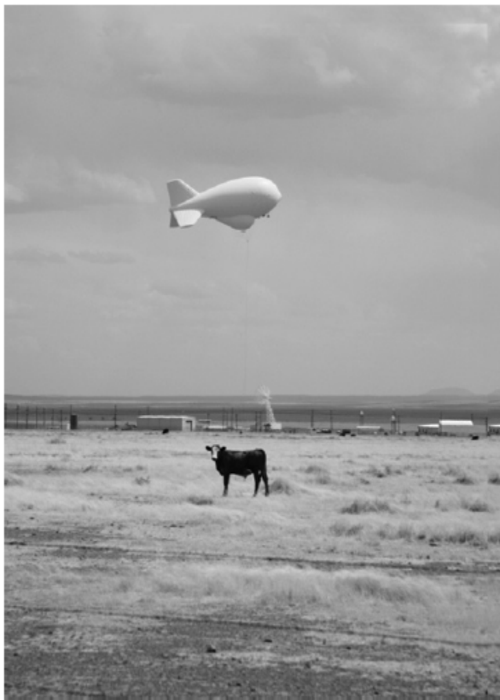
This Tethered Aerostat Radar System (TARS) near Marfa, Texas, provides drug interdiction radar surveillance. Balloons filled with helium tethered to a single cable serve as radar platforms. PHOTO: JOHNMCBRIDEPHOTOGRAPHY.COM
