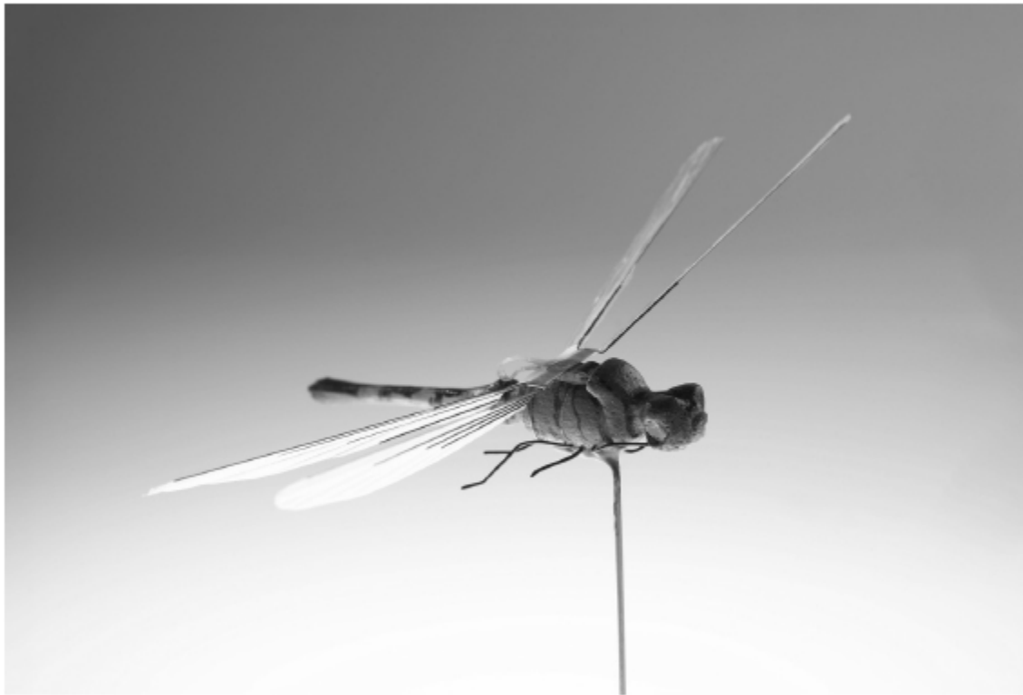
The CIA Office of Research and Development developed this Insectohtopter micro UAV in the 1970s as part of an initiative to explore intelligence collection by miniaturized platforms. CIA PUBLIC DOMAIN PHOTO
