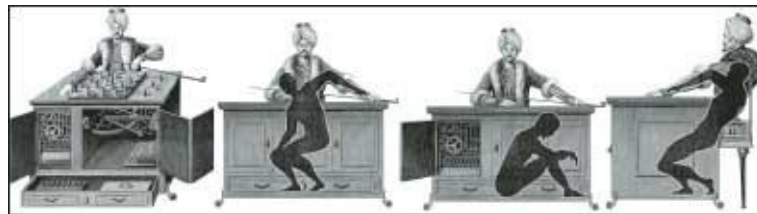
“Turk automaton.” The operator could hide under the shell of the automaton. (Illustrations by Victor Escandell for the Fundación “la Caixa” museum exhibit “Abracadabra, Ilusionismo y Ciencia”)
