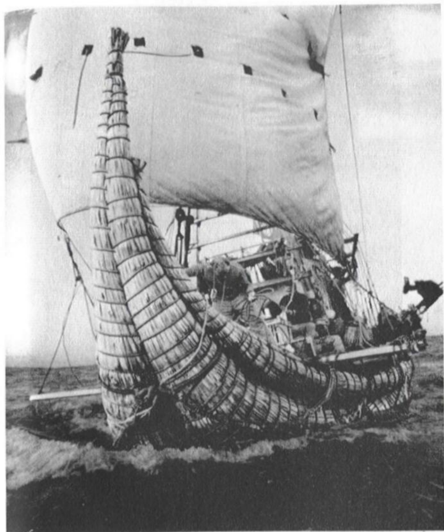
PLATE 12 Heyerdahl's Ra I, built by African boatmen. African boatmen from Lake Chad built this papyrus boat along the pattern of the ancient Egyptians. It left North Africa in 1969 and sailed as far as Barbados. Rudders broke early on the Ra , proving that an ancient drift journey in such a boat using Africa-to-America currents was feasible.
