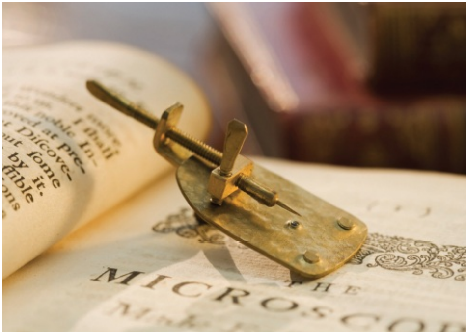
Antony van Leeuwenhoek's microscopes looked like glorified door hinges, but they were the best of his day and they allowed him to become the first human in history to see bacteria.
